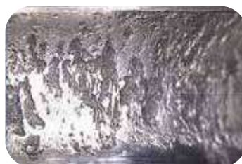
Bearing shaft race ways wear due to irregular loads applied to the water pump bearing
