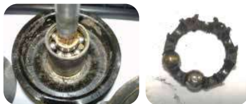
↕ Coolant has infiltrated inside the bearing removing it internal protective grease.
