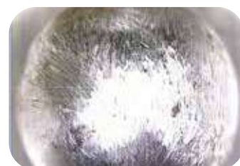
Typical wear produced by abnormal tensor movements due to incorrect tightening of screw that fix it.
