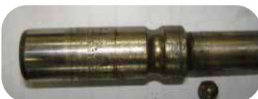
↕ Coolant has infiltrated inside the bearing removing it internal protective grease.
